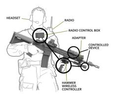
The RACU Hammer System consists of a finger/thumb operated Controller (the Hammer) attached to a GPS Grip-POD foregrip on the weapon, and a Radio Control Box (RCB) and cable assembly worn on the body. The Hammer sends commands either by cable or wirelessly to weapon-mounted and body-worn electronic devices.
