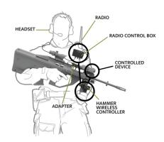
The RACU Hammer System consists of a finger/thumb operated Controller (the Hammer) attached to a GPS Grip-POD foregrip on the weapon, and a Radio Control Box (RCB) and cable assembly worn on the body. The Hammer sends commands either by cable or wirelessly to weapon-mounted and body-worn electronic devices.
